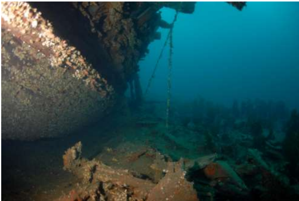
Fig. 5: View of the hull seen from forward port side, situation March 2012. It is very obvious that the planking below the former waterline has survived quite well. Along and above the waterline most of the hull planking has deteriorated (N. Mouchart).
