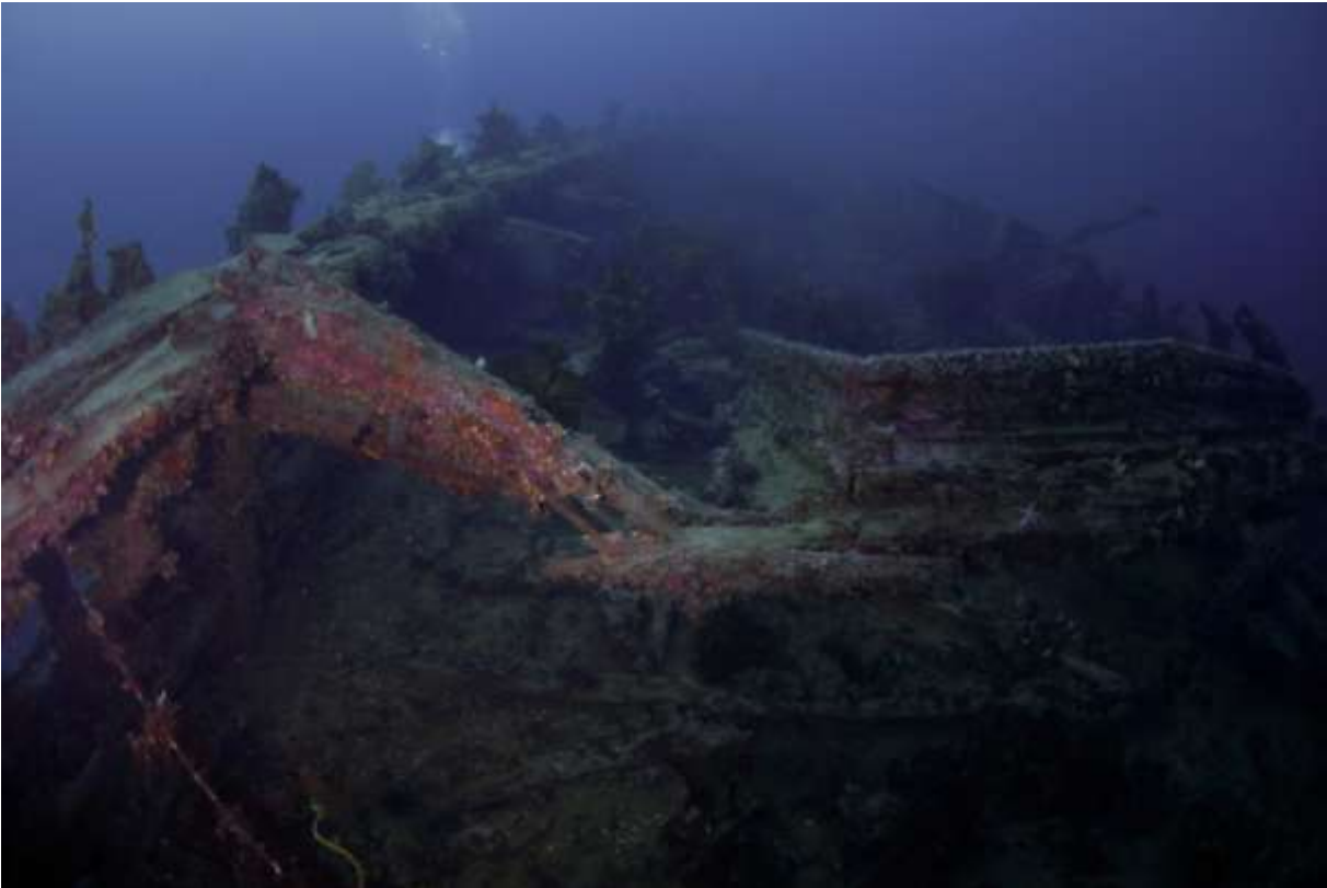
Fig. 13: View of the stern area, situation 2007. Part of the deck planking and fallen superstructure is still present on the top deck. This has all but disappeared and lies mostly scattered in the sand to port (N. Mouchart).
