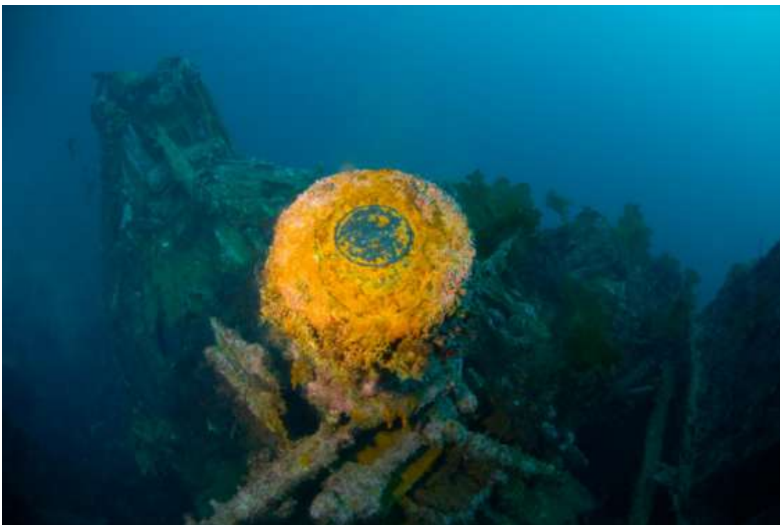
Fig. 3: Top view of the capstan, with the bow and the remains of the bowsprit in the left hand corner, situation March 2012. After 6 years the lettering on the cast iron capstan makers' plate have almost disappeared (N. Mouchart).
