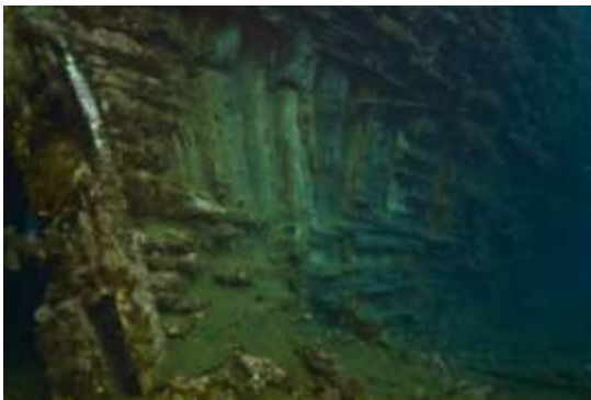
Fig 8: view of the stern, starboard side. Here the planking below the waterline has disintegrated (N. Mouchart).
