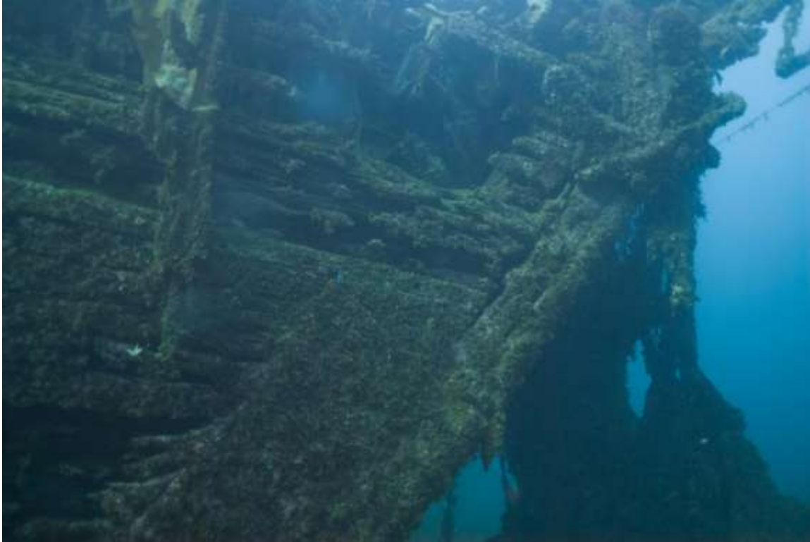
Fig. 2: View of the suspended starboard anchor, March 2012. Most of the of the hull planking above the waterline has disintegrated (Nicolas Mouchart).
