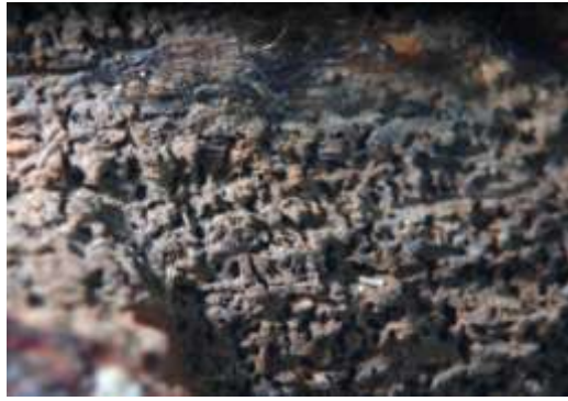
Fig. 7: One of the largest enemies of immersed wood: gribble, a wood boring crustacea (N. Mouchart).
